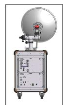
It is structurally composed of the following units: function generator, synthesized RF generator with internal variable attenuator, SSA type power amplifier, transmitting antenna, DC / DC converter for system power supply, batteries and charging circuit and mechanics support including antenna support and wheels for handling the system.
